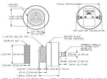
NOTE A: TERMINALS-032 BRASS TIN PLATED, TAPPED FOR #6-32 SCREW, TWD #6-32 NICKEL PLATED BRASS SCREWS INCLUDED, WILL ACCEPT 1/4\* QUICK CONNECT.
