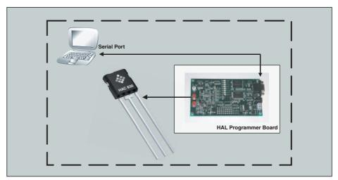
Fig. 1: Development tool setup
