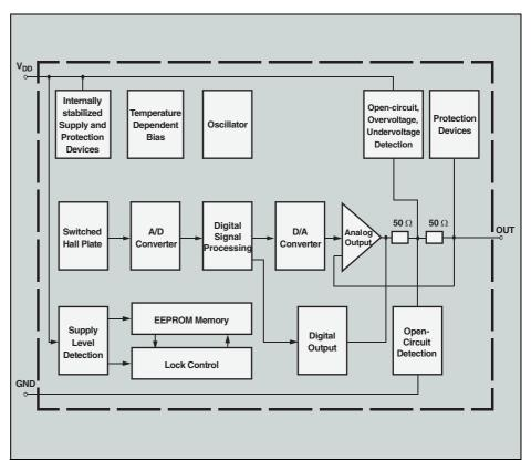
Fig. 2: Block diagram of the HAC 830
