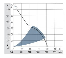
Air performance measured according to: ISO 5801. Installation category A, without contact protection. Noise: Total sound power level  $L_WA$  ISO 103002 measured on a hemisphere with a radius of 2 m. Sound pressure level  $L_PA$  measured at 1 m distance from fan axis. The values given are applicable only under the specified
