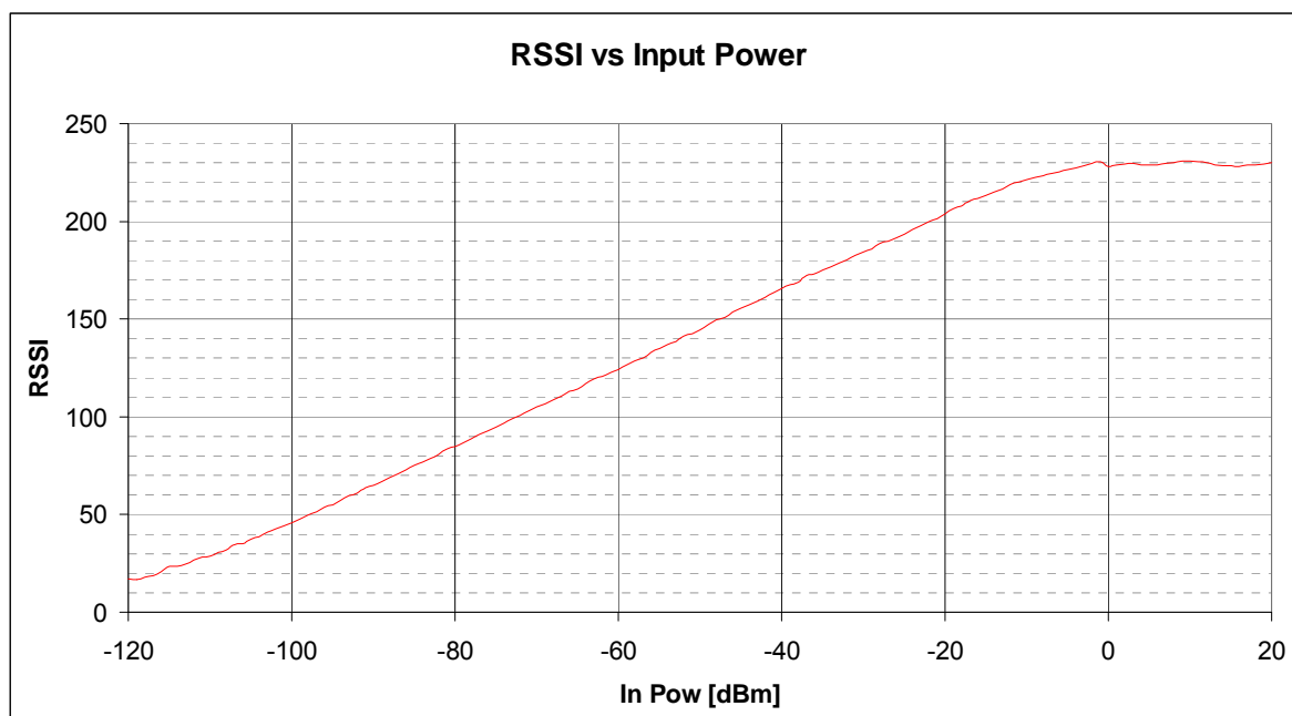
Figure 31. RSSI Value vs. Input Power
