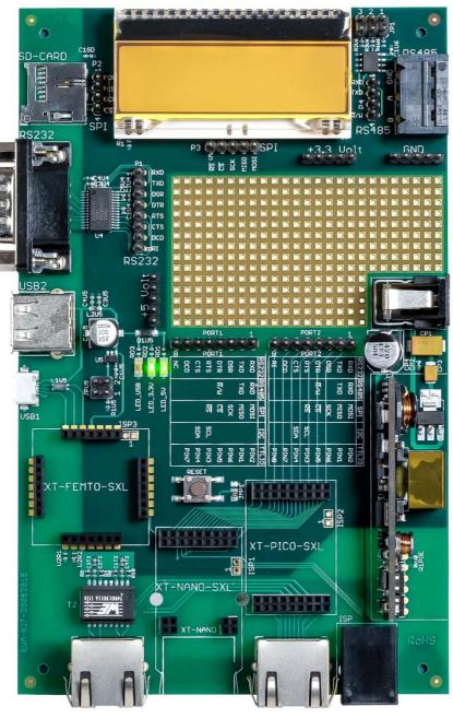
XT-FEMTO XT-NANO XT-PICO DEBUG slot slot slot connector
