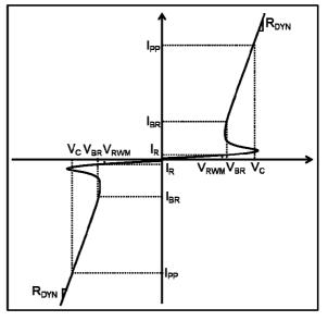
Fig. 7.1 Definitions of Electrical Characteristics
