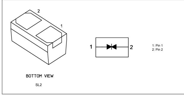
Note: Connect Pin 2 to GND when using Pin 1 for I/O. Connect Pin 1 to GND when using Pin 2 for I/O.
